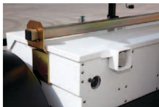
Secure battery box
