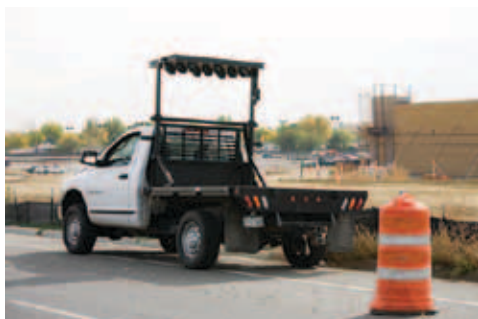
Arrow board with 90° power-tilt frame in travel position
