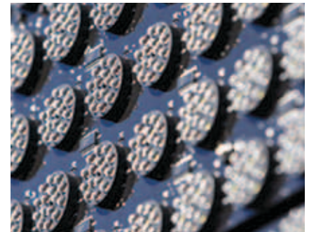
15 LEDs per pixel, 3 of each color
